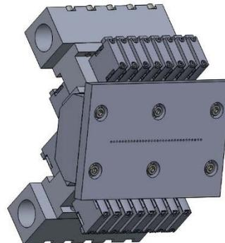
Figure 2-2. Airjet manifold for sorting system.
