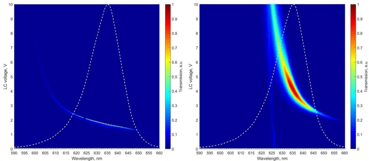
Figure 5-2. Left | Spectral response of an LCAM with craters ablated into one of the mirror surfaces. FSR= 58.5 nm,  $\Delta\lambda=53$  nm, FWHM < 1 nm | Spectral response of an LCAM with no craters. FSR=80nm,  $d_l=55$ nm, FWHM > 3.6nm. The white dotted lines show the spectra of the unfiltered LED light that is incident on the LCAM.
