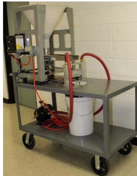
Figure 2-1. Shaker feeder on steel cart
