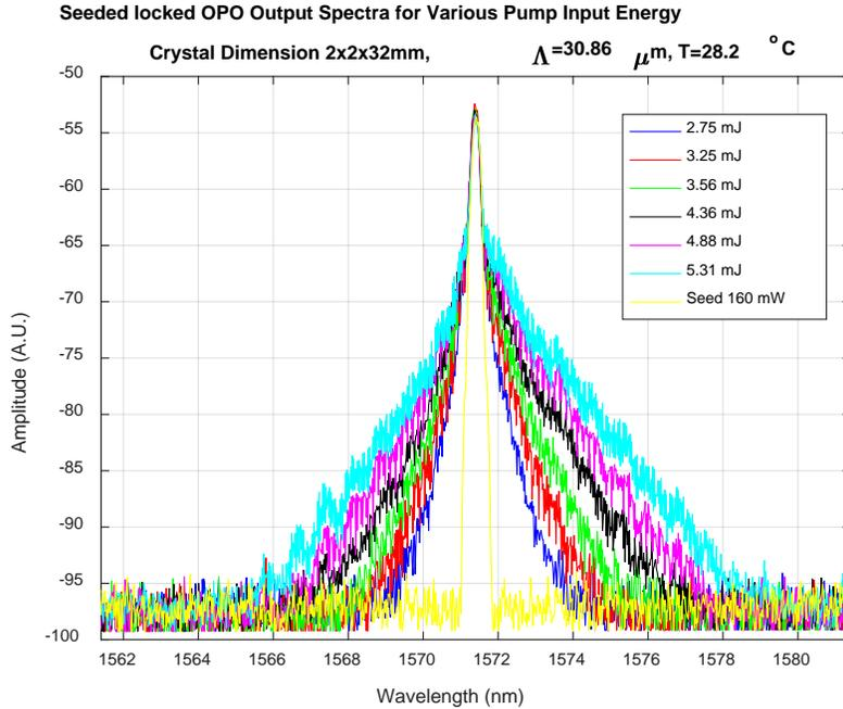
Figure 9-8. Output spectra for seeded-locked OPO.
