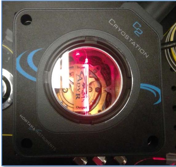
Figure 8-10. Example of optical fiber coupling of AdvR Inc waveguide within a Montana Instruments Cryostation.
