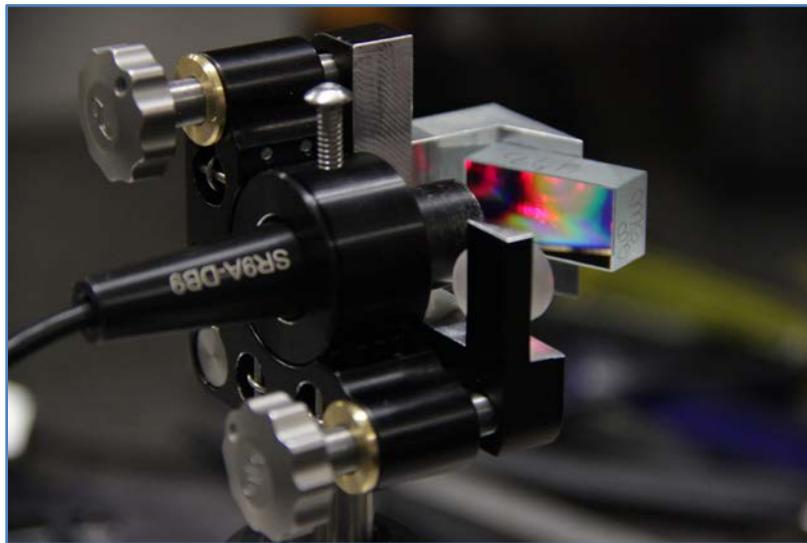
Figure 8-12. Simple and inexpensive tunable diode laser system constructed at MSU to enable new research and applications employing regions of the optical spectrum that have not been previously accessible for rare-earth-activated devices.
