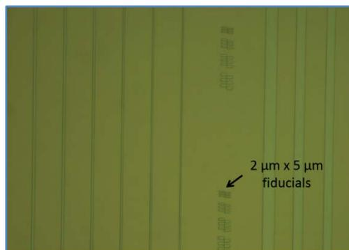
Figure 8-3. Microscope image of optical waveguides. The 2 μm fiducials are used to visually determine the quality of smallest fabricated waveguide diameter.
