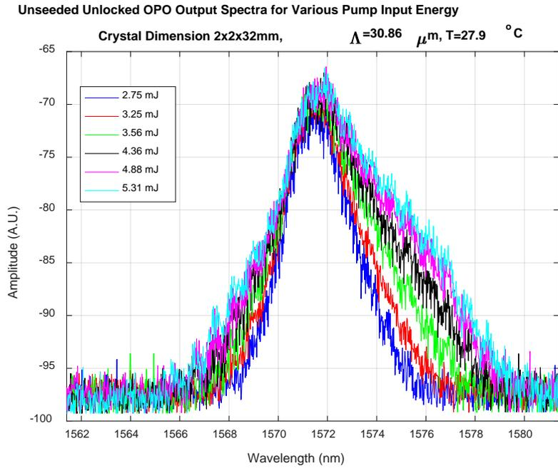
Figure 9-6. Output spectra for unseeded-unlocked OPO.
