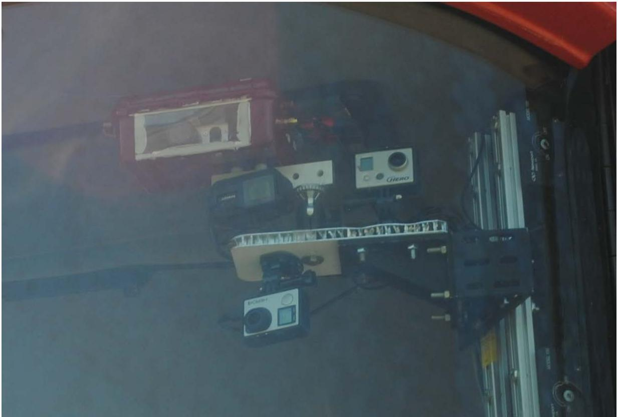
Figure 1-1. Imaging systems mounted inside the combine cab with 5 different cameras.
