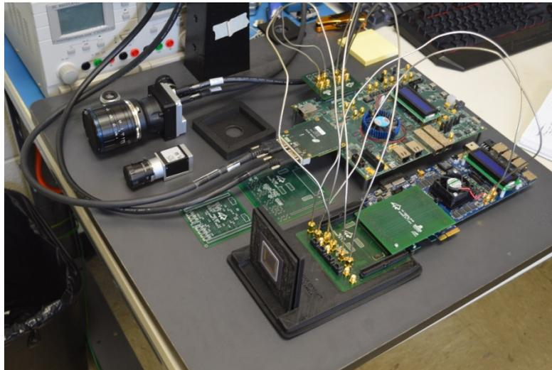
Figure 2-4. High-speed serial links between Arria V FPGA board and Arria 10 FPGA board.
