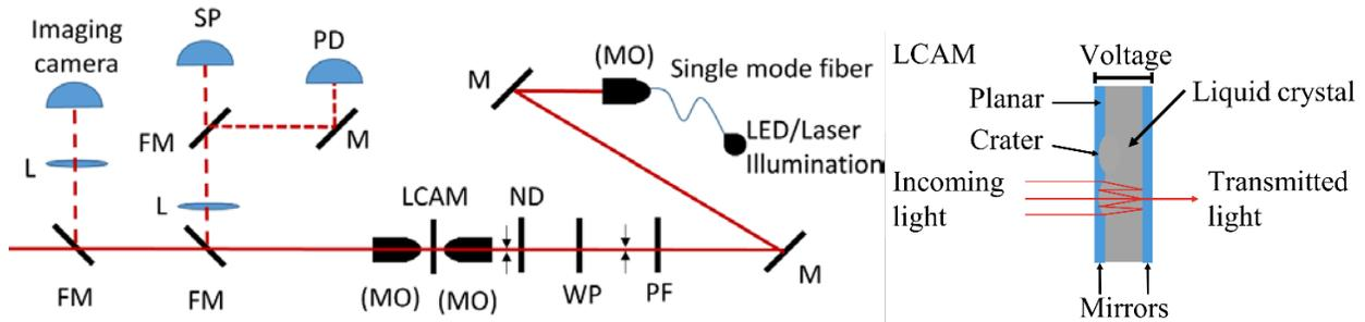
Figure 5-1. Left | Schematic of the LCAM characterization testbed. M-Mirror, MO-Microscope objective, FM-Flipper mirror, WP-Wave plate, ND- Neutral density filter, PF-Polarizing film, SP-Spectrometer, PD-Detector, L-Lens. Right | Schematic of a LCAM optical filter.
